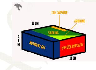
The packet in the box includes nutrient gel, sapling, Arduino board (microcontroller), and carbon dioxide cartridge.
